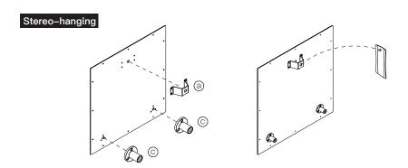
Align (a) and (b) to the hole position of aluminum alloy decorative panel, and use (d) to lock, then hang on 3M metal hook to complete the installation.
