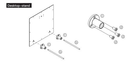
Aligned 0 to the hole position, slightly lock the 0 on the back of the aluminum alloy decorative panel and insert 0 into 0 to complete the installation.
